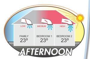
Using the Platinum II Zone Control System, wireless sensors measure temperature in individual rooms, dampers adjust automatically and airflow is redistributed in order to maintain a constant temperature. Dampers can also be adjusted manually to suit personal preferences for individual rooms.
